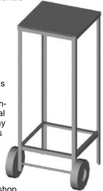
An existing table could be retrofitted, if you have access to a shop and a welder. Two of the legs could be shortened and fitted with a steel rod, two lawnmower wheels (about \$7.50 each), and push-on retaining caps, all of which are available at hardware stores.
